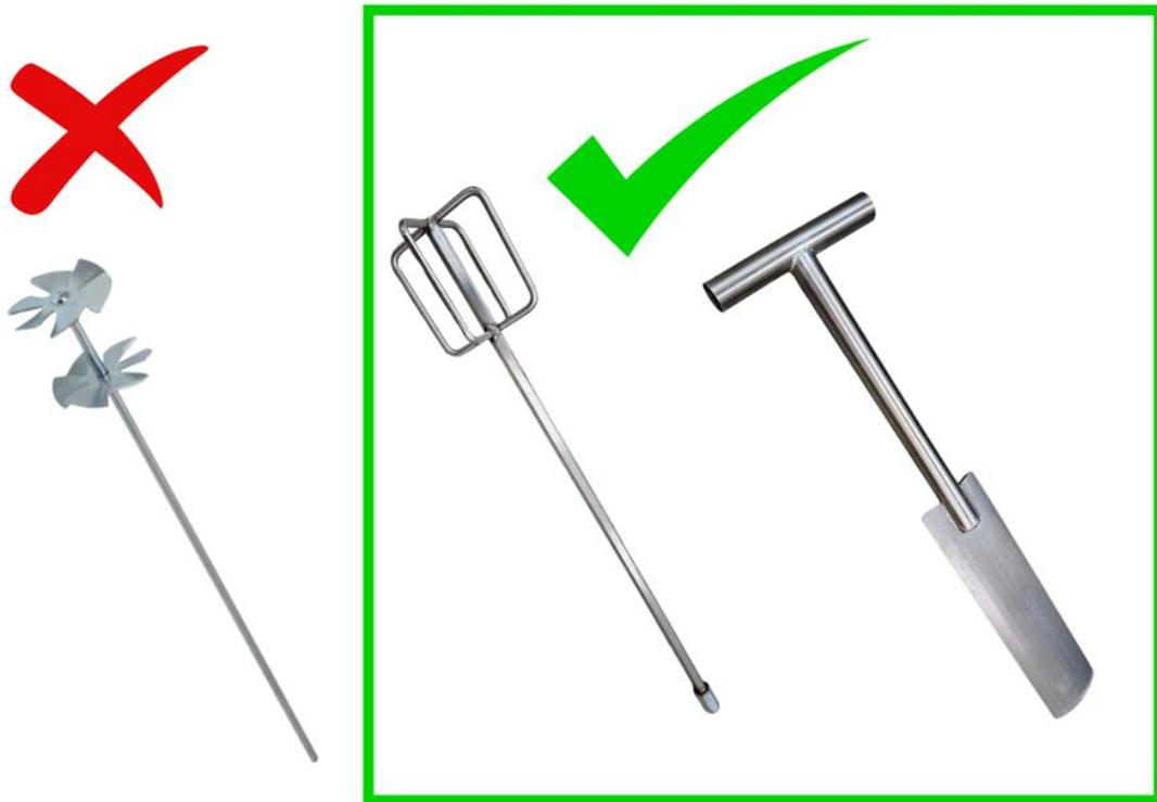
A drill-operated stirrer must not have sharp edges because these will scrape plastic shards off the bucket which will end up in the coating.
