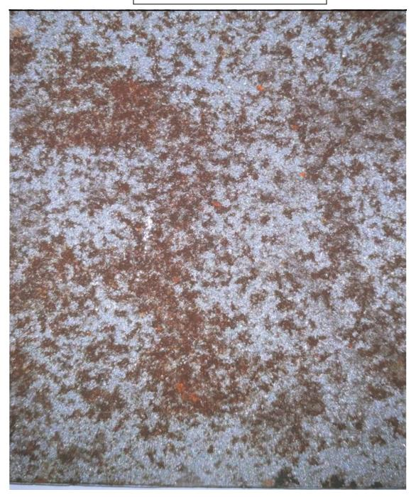
NOT ACCEPTABLE This surface is covered in mill scale. This is a very unreactive form of oxidation – Fe304. No coating should be applied on mill scale.
