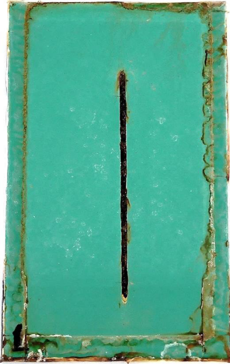
Sample Panel #1 - Dark Green at 12 Cycles Exposure IAW ASTM D5894-16 (see above)
