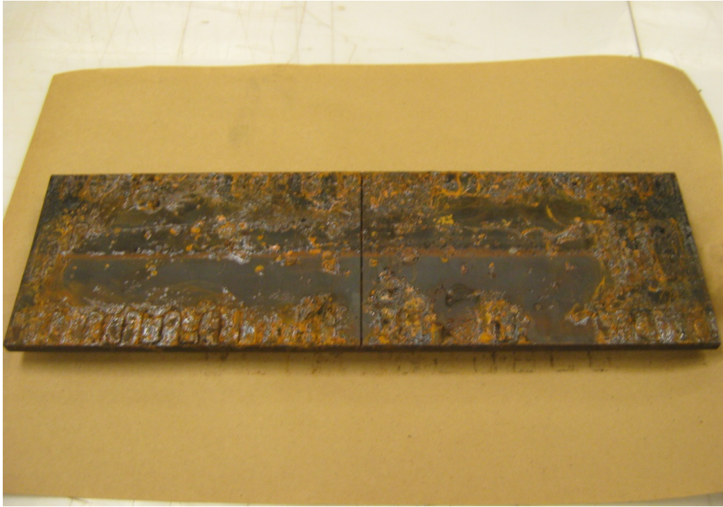
Figure 35. Drip Zone Bottom Surface after 3 Weeks
