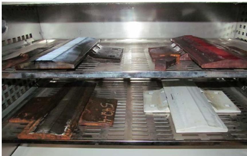
Figure 10. Placement of Samples in Humidity Cabinet
