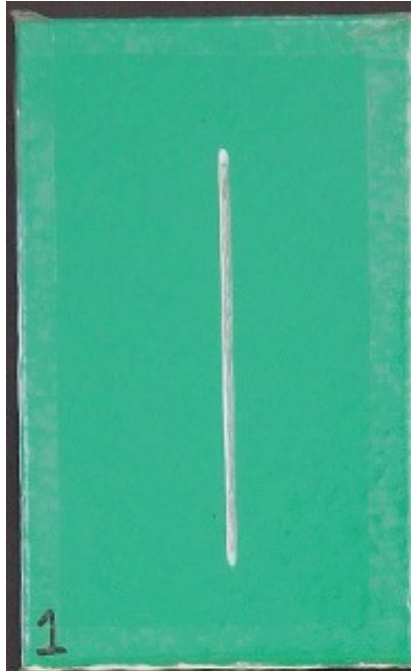
Sample Panel #1 - Dark Green prior to Exposure IAW ASTM D5894-16 (see above)
