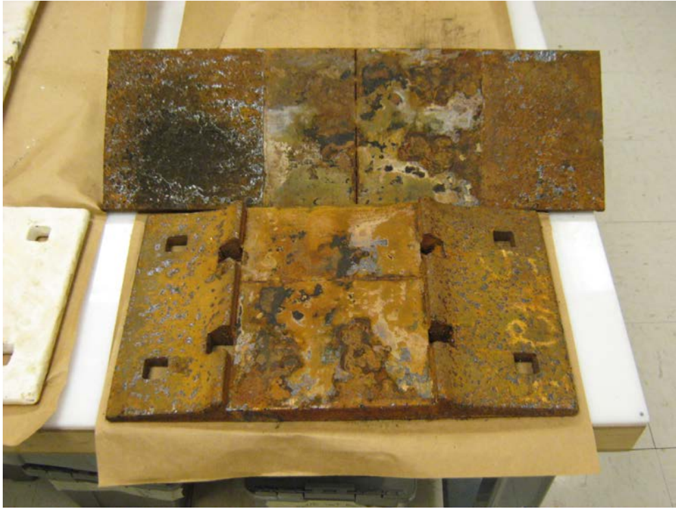
Figure 32. Untreated Samples after 3-Week Exposure
