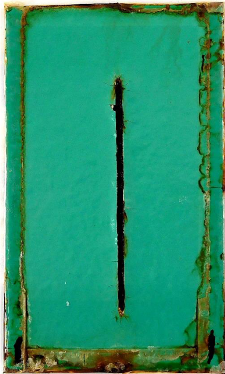
Sample Panel #1 - Dark Green at 15 Cycles Exposure IAW ASTM D5894-16 (see above)
