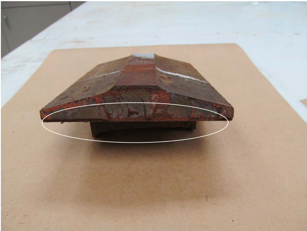
Figure 40. Fracture Surface of Corroded Sample with No Protection (Crack – corrosion area is circled)
