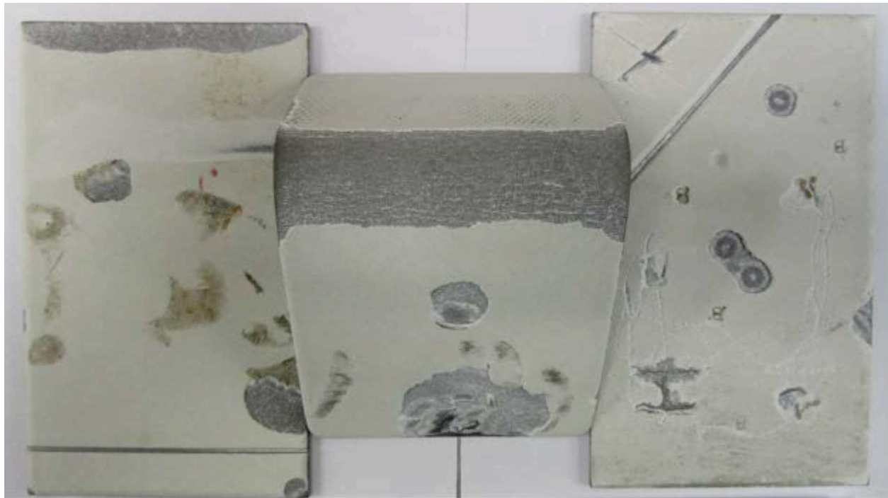
Figure 1 – EonCoat panels with intentional mechanical damage.
