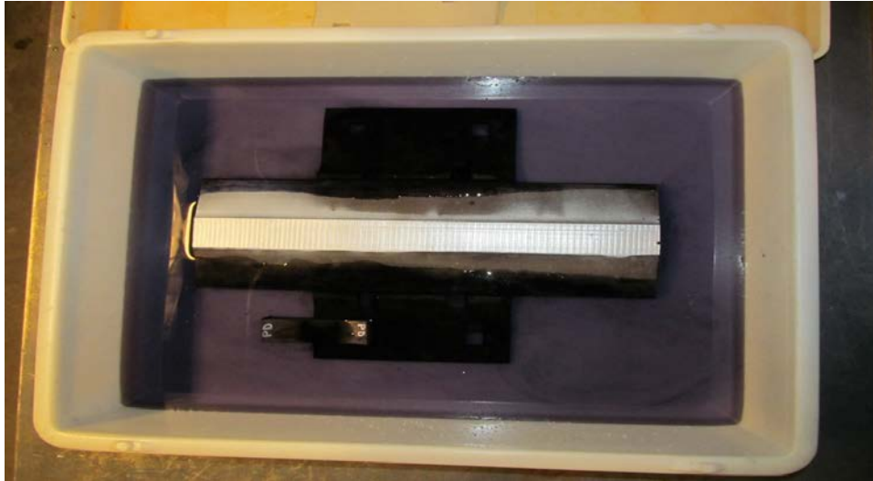
Figure 9. PD Samples on First Exposure to Saltwater
