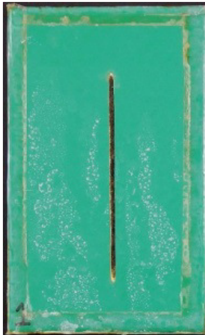
Sample Panel #1 - Dark Green at 3 Cycles Exposure IAW ASTM D5894-16 (see above)
