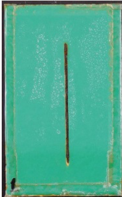
Sample Panel #1 - Dark Green at 6 Cycles Exposure IAW ASTM D5894-16 (see above)
