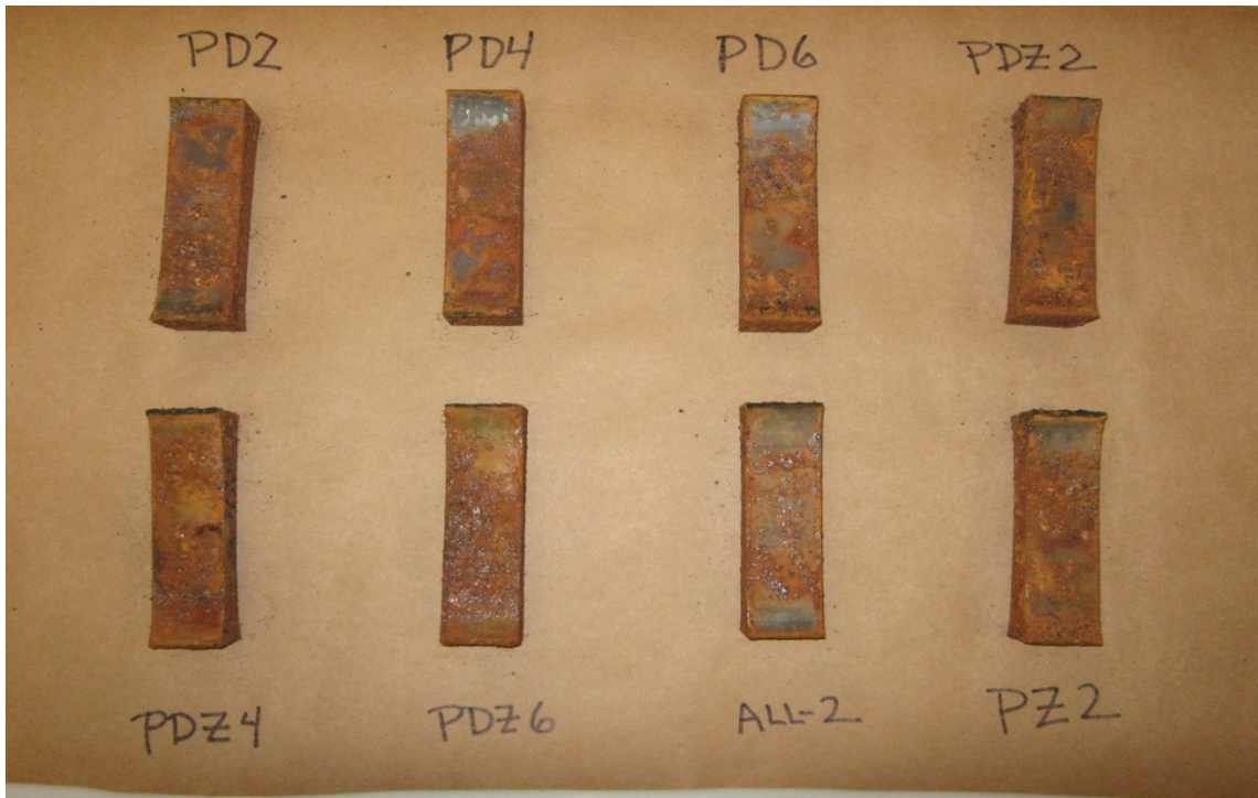
Figure 17. Bottoms of Samples after 3-Week Corrosion Cycle
