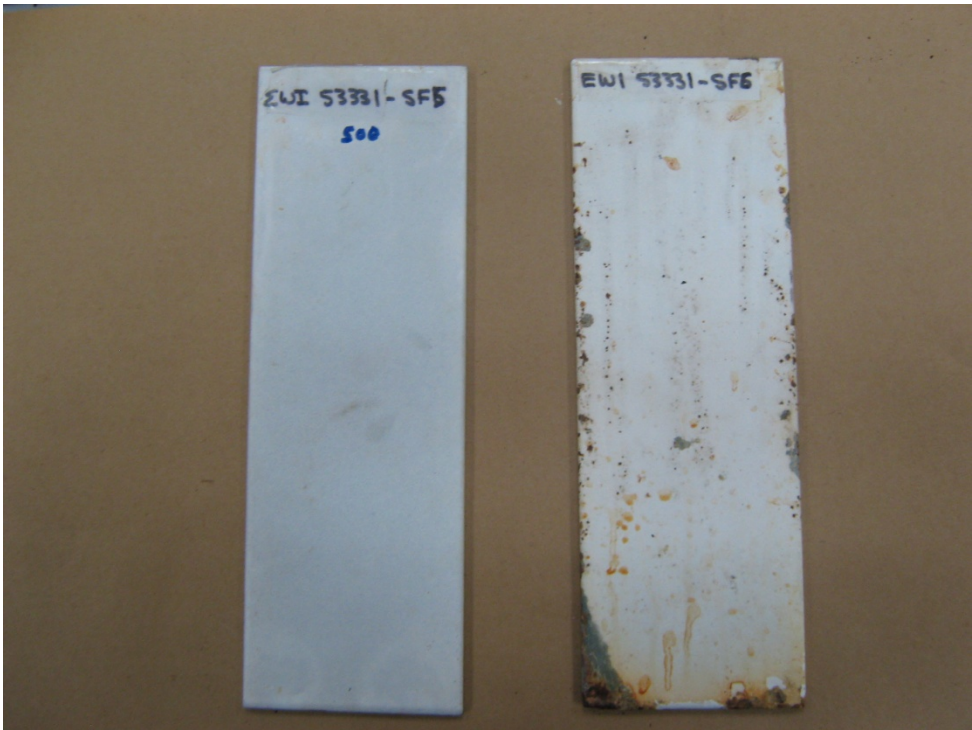
Figure B-5. EonCoat®, Back Side. L→R: 500, 1500 Hours
