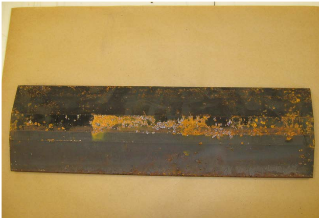
Figure 34. Drip Zone Top Surface after 3 Weeks
