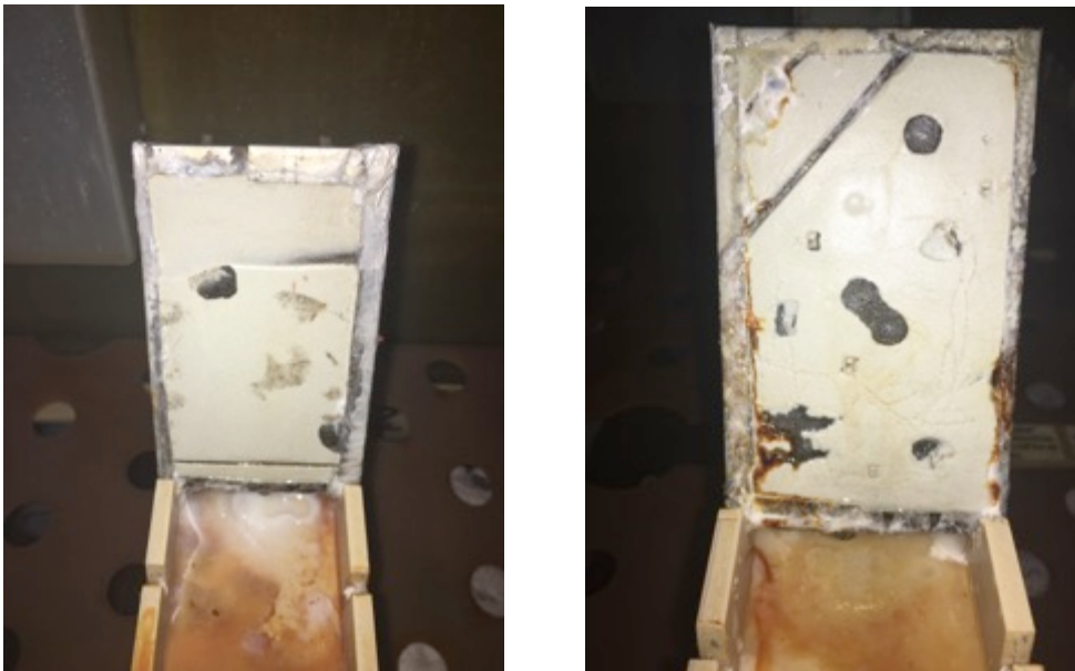
Figure 3 – EonCoat panels with intentional damage after 1,870 hours of B117 exposure.
