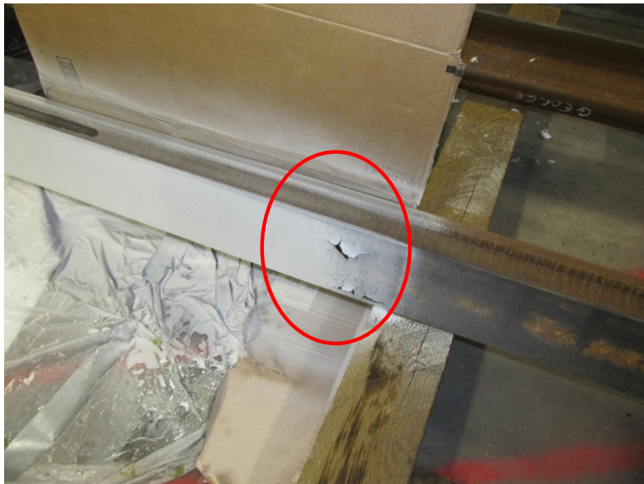
Figure 15. EonCoat® Sprayed Rail Segment
