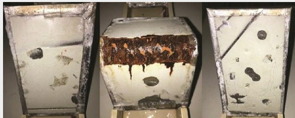
Panels with intentional damage after 335 h of ASTM B117 exposure. Photo courtesy of EUROCORR 2018.
