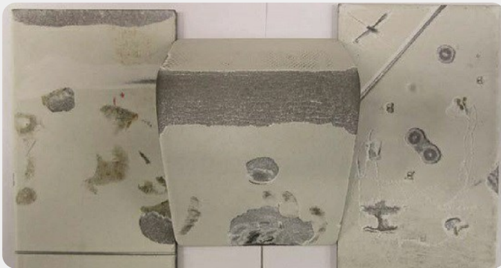
Sample panels with intentional mechanical damage. Photo courtesy of EUROCORR 2018.
