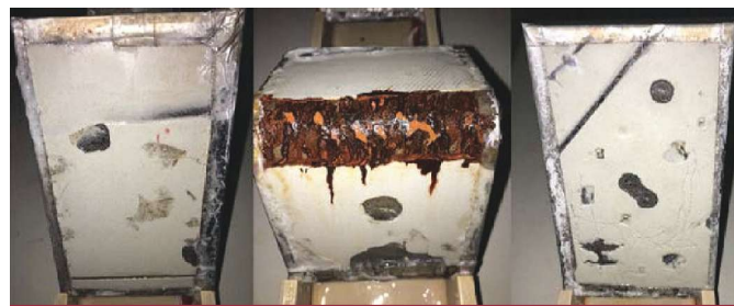
Panels with intentional damage after 335 h of ASTM B117 exposure. Photo courtesy of EUROCORR 2018.
