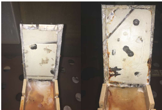
Panels with intentional damage after 1,870 h of ASTM B117 exposure. Photo courtesy of EUROCORR 2018.
