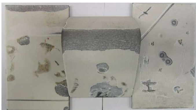
Sample panels with intentional mechanical damage. Photo courtesy of EUROCORR 2018.
