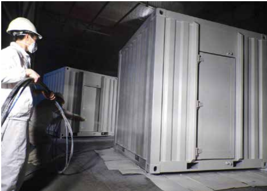
In contrast to additional polymer coatings that sit on top of the substrate, the corrosion resistant CBPC coating bonds through a chemical reaction with the substrate, and slight surface oxidation actually improves the reaction.
