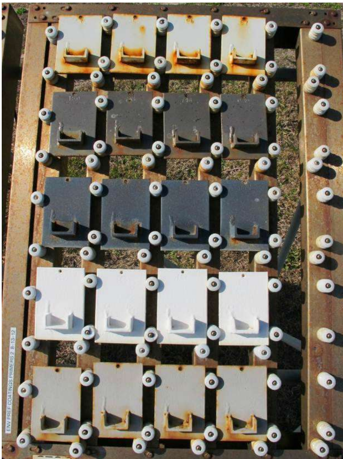
Figure 18 Systems 6-10 Primer-only Test Panels – 6 Months (02/13/2013)
