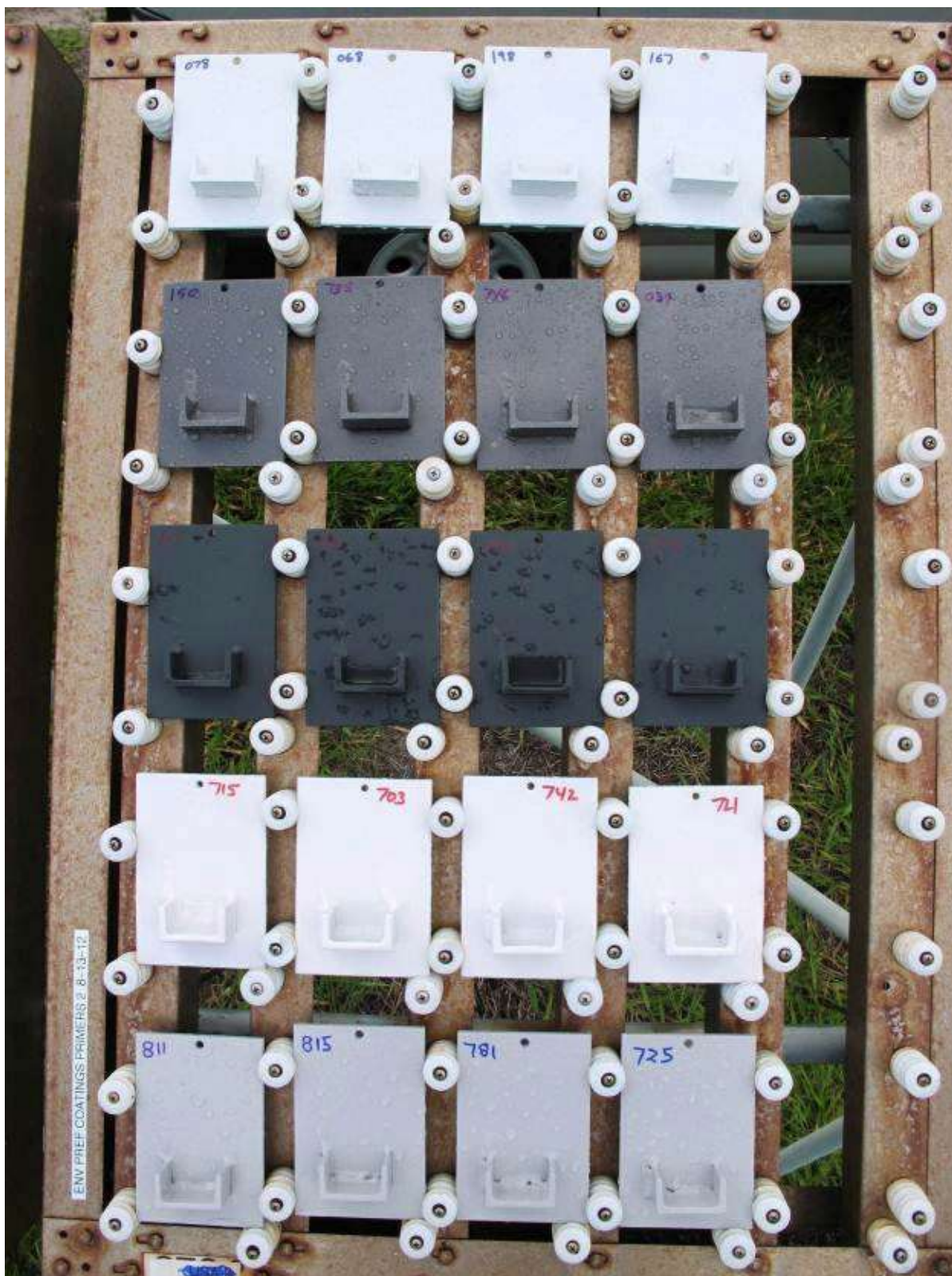
Figure 17 Systems 6-10 Primer-only Test Panels – Initial (08/13/2012)
