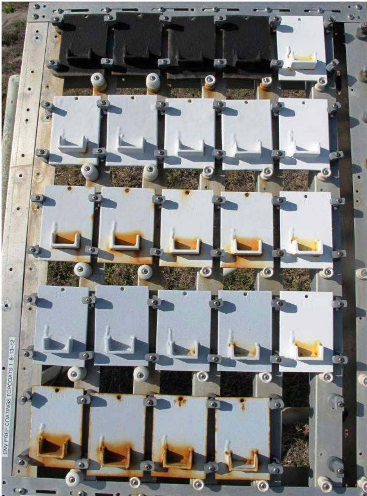
Figure 23 Systems 1-5 Full System Test Panels – 6 Month (02/13/2013)
