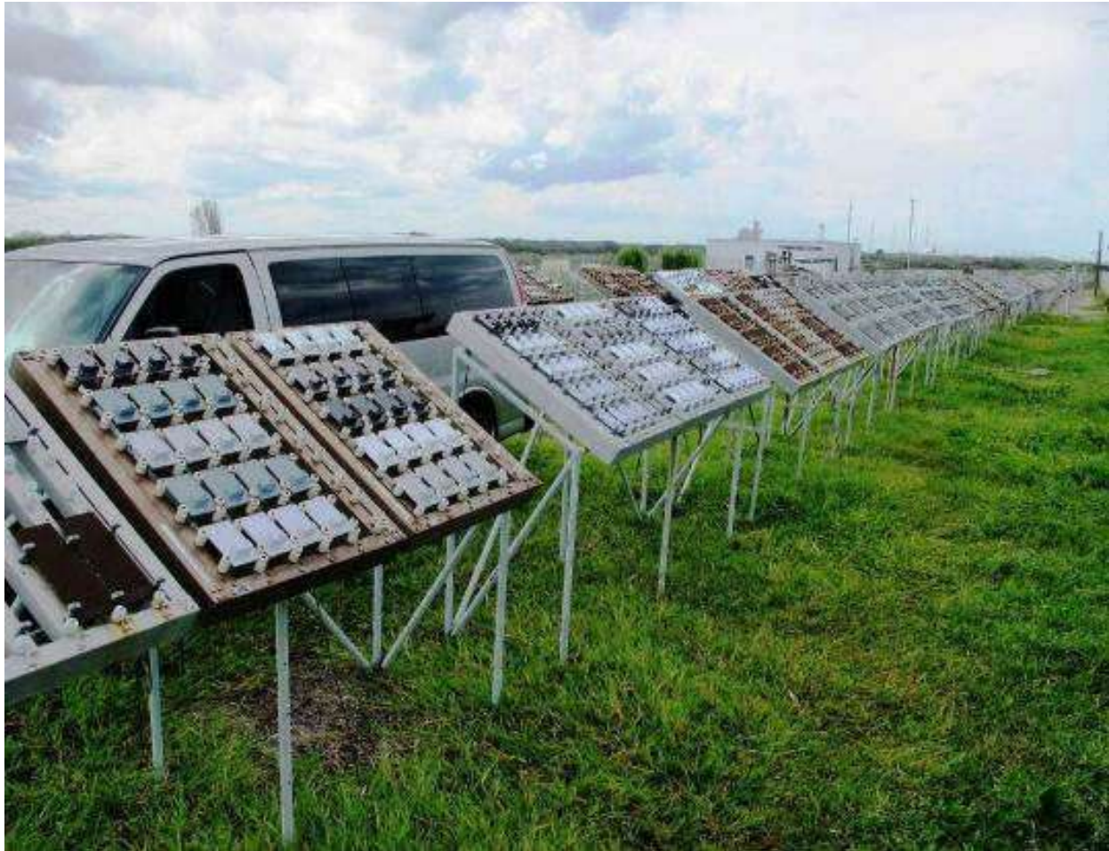
Figure 6 KSC Beachside Atmospheric Test Facility Test Racks
