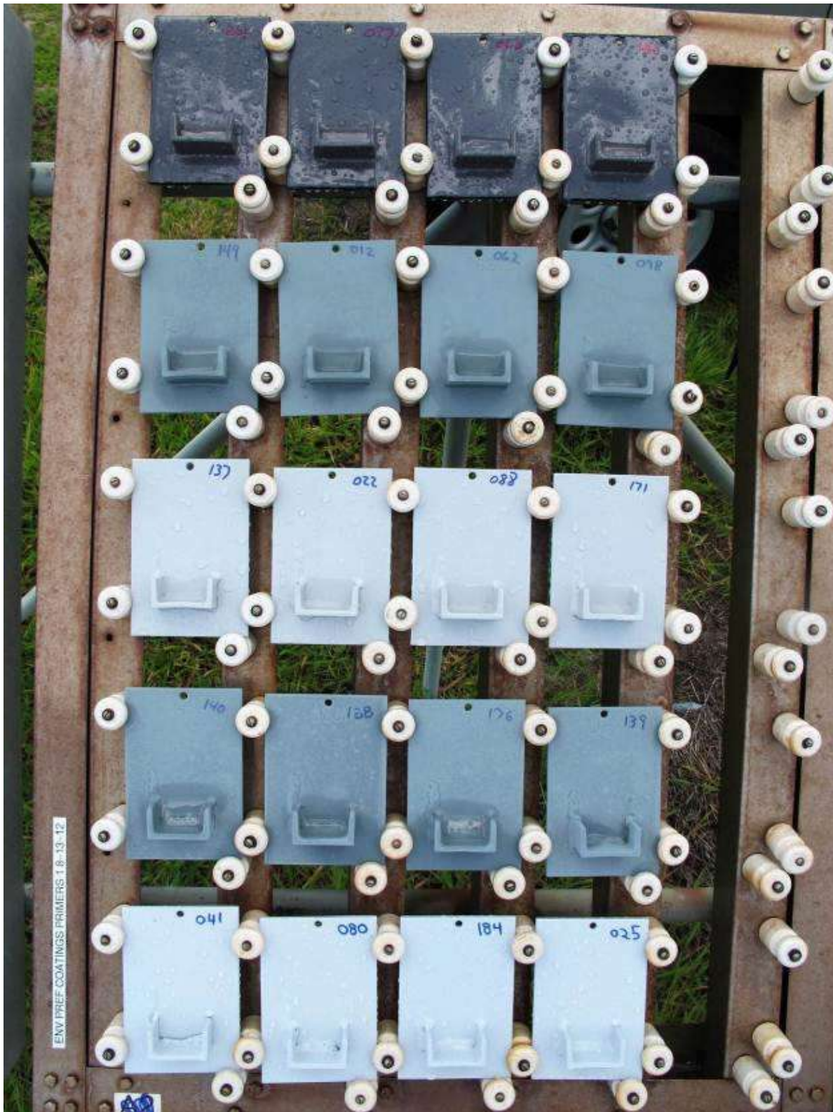
Figure 12 Systems 1-5 Primer-only Test Panels – Initial (08/13/2012)
