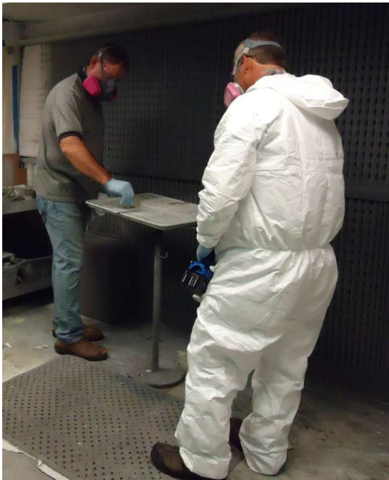
Figure 3 Quality Control Check during Application of Alternative Coating to Test Panel
