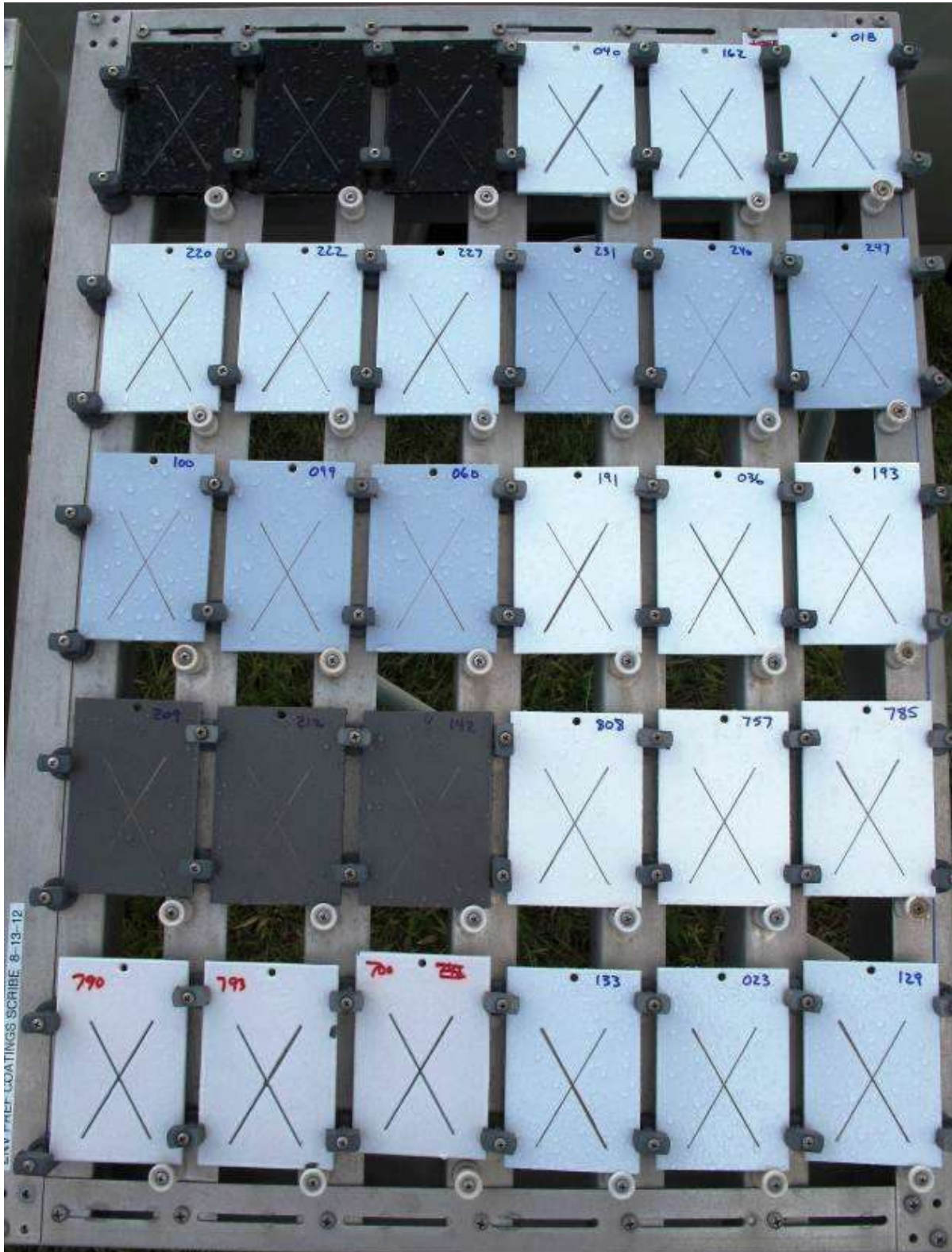
Figure 32 Full System Scribed Test Panels – Initial (08/13/2012)
