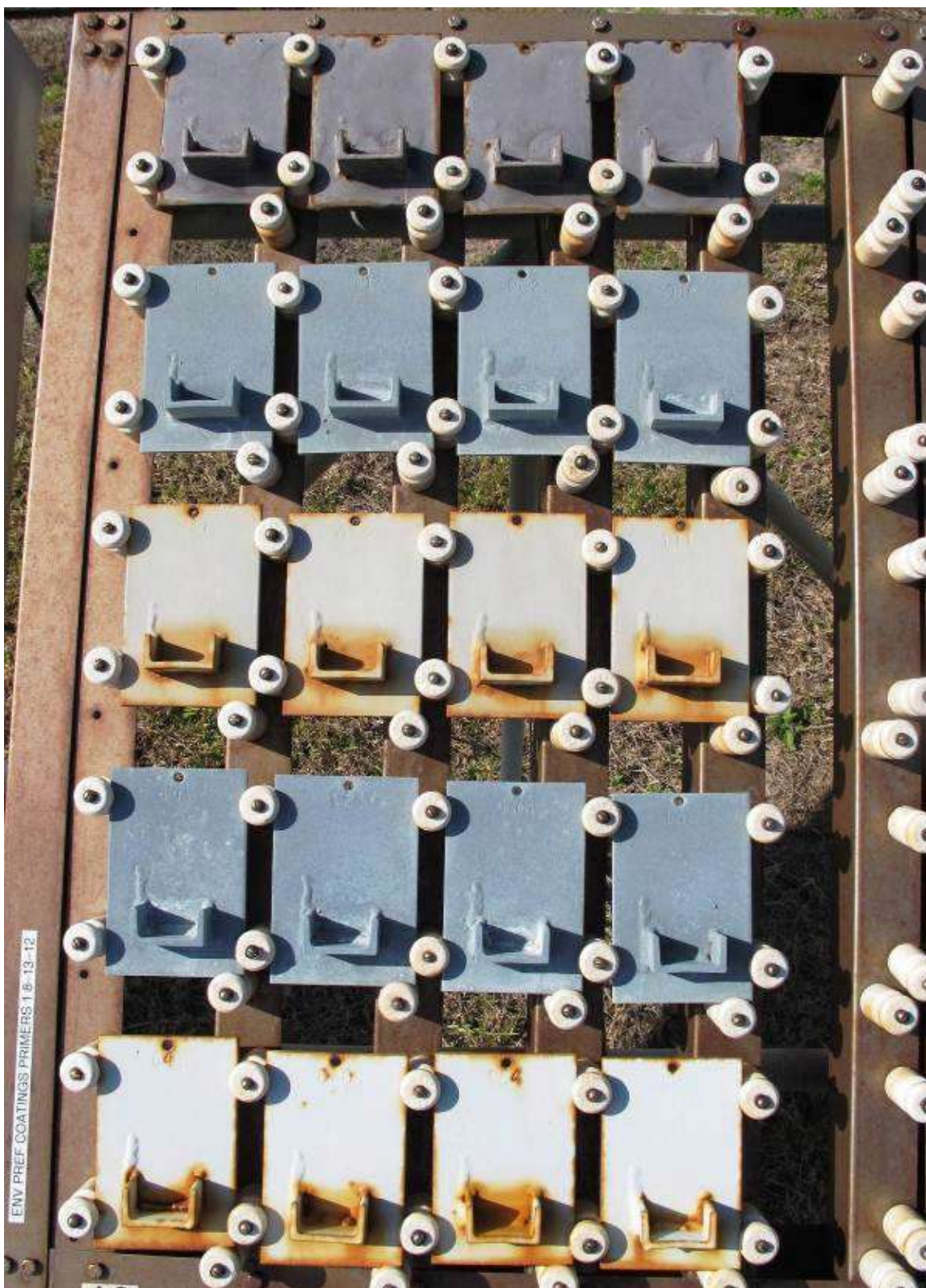
Figure 13 Systems 1-5 Primer-only Test Panels – 6 Months (02/13/2013)
