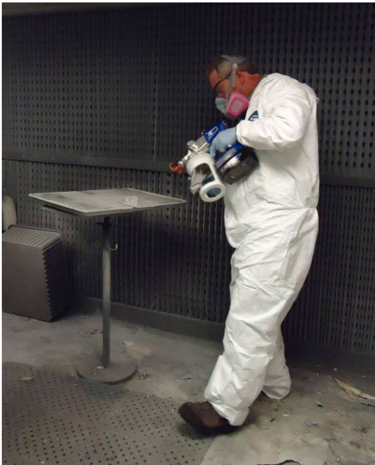
Figure 2 Application of Alternative Coating to Test Panel
