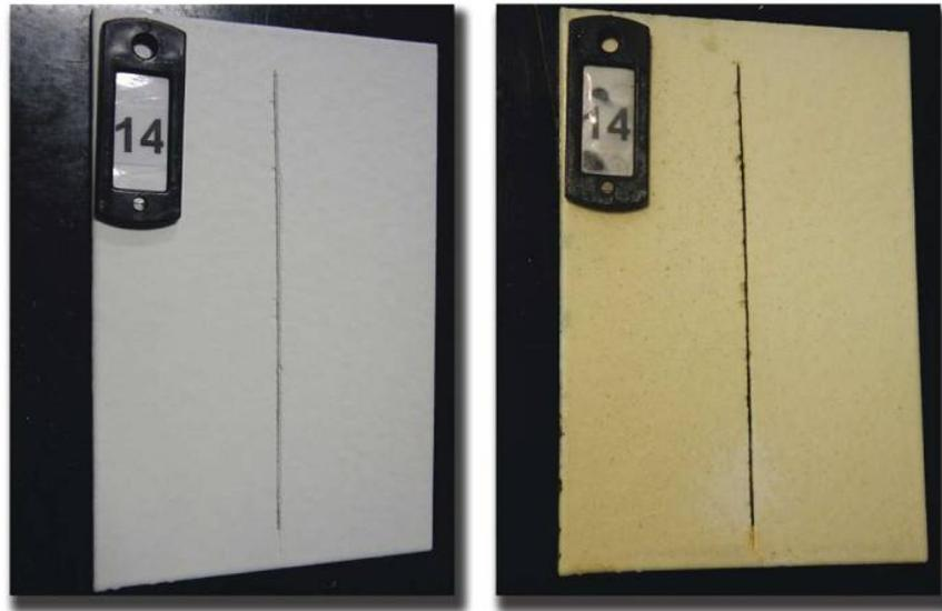
The photos show a steel sample coated with the protective CBPC coating on the first day of a NASA-developed seawater corrosion test (left) and after 170 days of continuous exposure (right). Photo courtesy of EonCoat.
