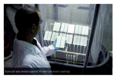
a corrosion-resistant passivation layer of iron oxy hydroxide. Because the passivation layer is electrochemically stable, like gold and platinum, it does not react with corrosion promoters such as water and oxygen."
