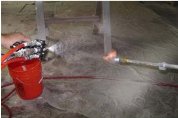
EonCoat has a flame spread rating of zero which can help prevent flame spread on coated walls, ceilings, equipment, cargo holds or wherever a fire barrier is needed.
